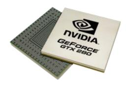
between, where we can exploit the advantages of each. The current performance part has 240 processors running at 1.3 - 1.6 GHz. With dual-issue capabilities, this places the peak performance over 1 TFLOP. CUDA is the C programming language with a few extensions for programming the Tesla chips. These include thread launch/terminate, synchronization, sharing, and atomic operations.
